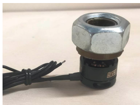
(c) M14 metric nut mounted to threaded flywheel attached with motor manufacturer’s prop shaft and bolt.
