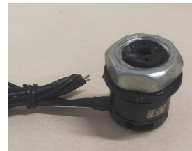
(b) M12 metric nut mounted to threaded Ninjaflex filament flywheel.
