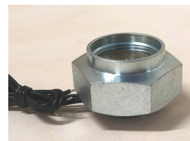
(d) M28 metric nut mounted to threaded flywheel press-fit over the brushless motor.
